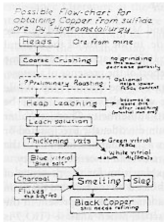
Figure 3. Possible flow chart of byproduction of green vitriol in the heap-leaching process. (Reprinted, with permission, from Koucky and Steinberg [1982: 168]; copyright 1982, Smithsonian Institution Press.)
