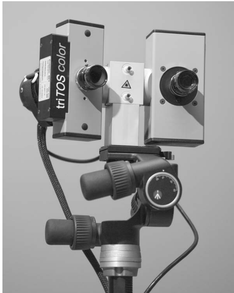
Fig. 4. Breuckmann triTOS-HE structured light scanner on tripod head, showing projector and camera components, with 10cm sensor bar between
