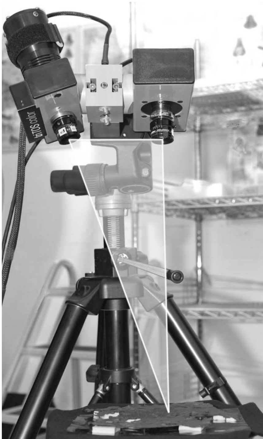
Fig. 5. Breuckmann triTOS-HE structured light scanner in use, 20° triangulation. Lower point of triangle represents one of a million points typically collected in this 10cm field of view. Object is identified in fig. 9
