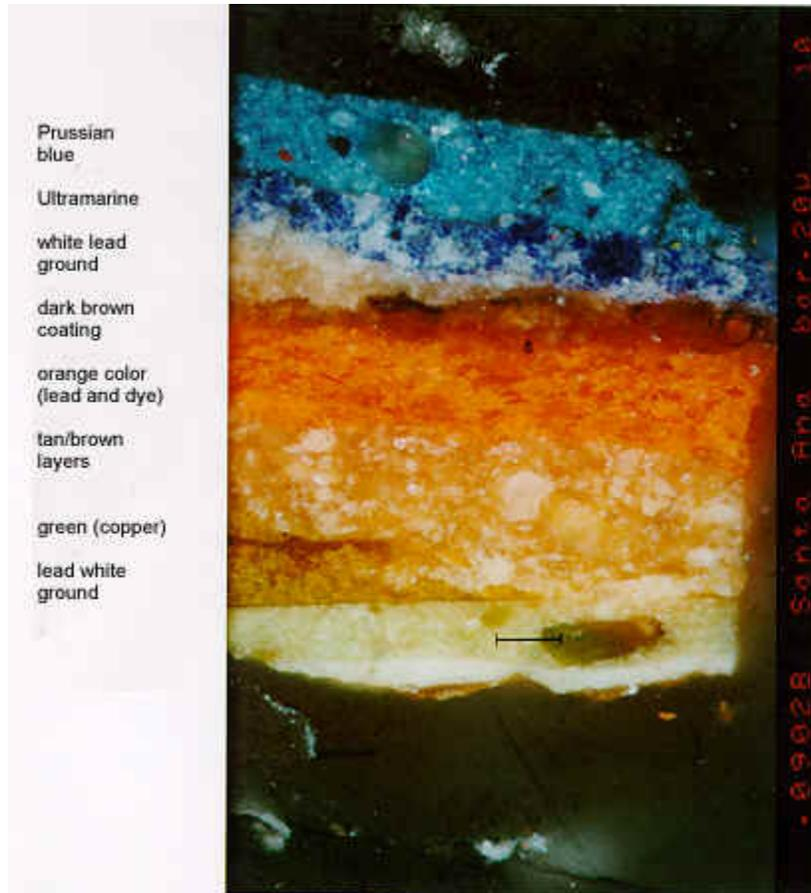
(Figure N) Paint cross-section from *Santa Ana's* blue robe.
