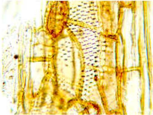
(Figure B) Tangential section from *Santa Rosalia* showing inter-vessel pits.
