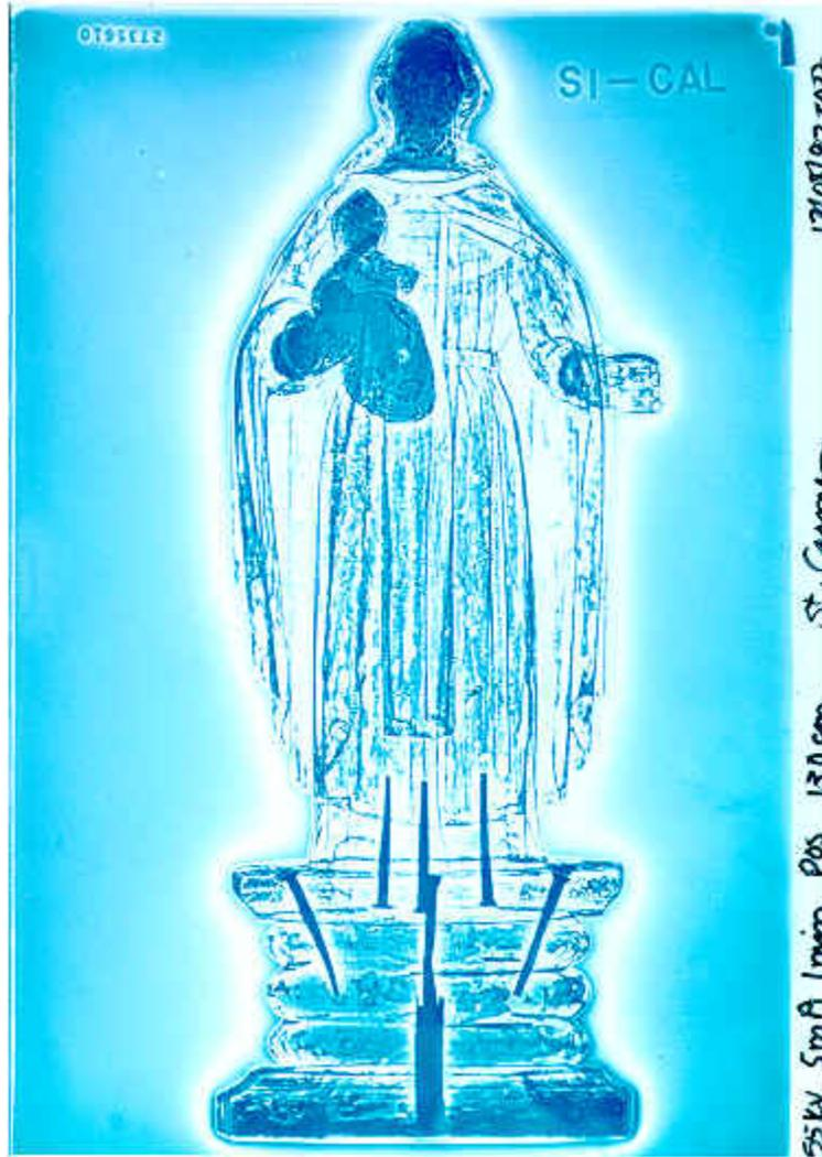
(Figure F) Xeroradiograph of *Virgen del Carmen*. The *Virgen's* face and the child are made of wax and appear dark. The xeroradiograph reveals how the stand is attached to the statue with nails.
