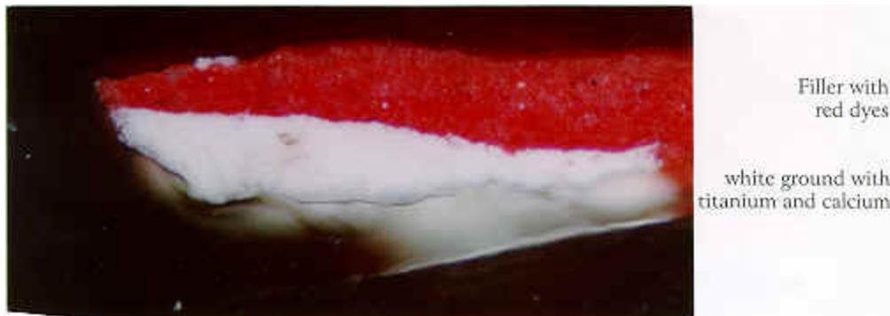
(Figure Z) Cross-section from the undercut of the red cape.
