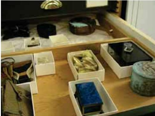
Acid vapors released from degraded plastic materials (center) have corroded a metal pan (center top) and a metal box (lower right) in same drawer. Domestic Life Collections at NMAH photo credit Preservation Service, NMAH
