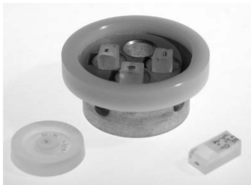
Fig. 2. Epoxy disc (left) and tablet (right) embedding forms, with holder for preparation and examination of four tablets. Preparation time is greatly reduced by mass production, but benefits are found in the application of principles to single samples (left).
