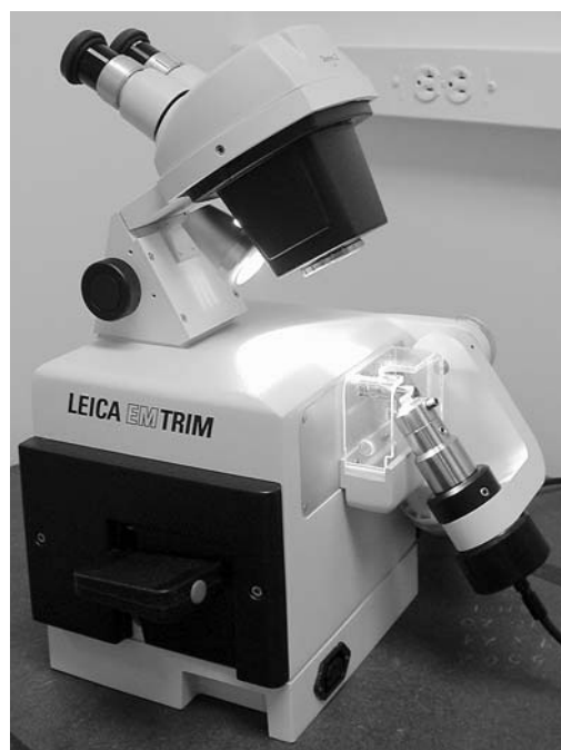
Fig. 16. Leica EM Trim used for ultramilling. This machine allows rapid exposure of the sample with great control.
