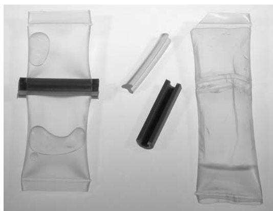
Fig. 7. Epoxy is mixed by sliding off center clamp (at left: catalyst in top portion, resin below); two-piece sliding clamp at center; corner cut open for pouring after mixing (small hole functions as dropper); unused resin allowed to harden prior to disposal.
