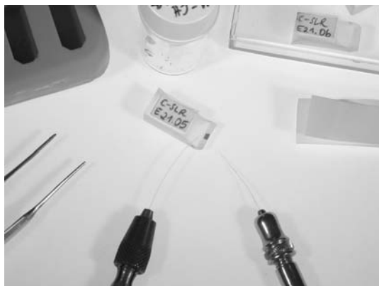
Fig. 4. Essential materials for embedding, with tablet with sample on shelf at center. Clockwise from top center: samples in vial, labeled half-tablets ready to mount samples, adhesive-backed label paper, needle holders with fishing-line probes, tweezers, commercial mold for final casting
