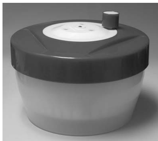
Fig. 24. Kitchen fruit and vegetable spinner serves as an inexpensive, highly effective centrifuge.
