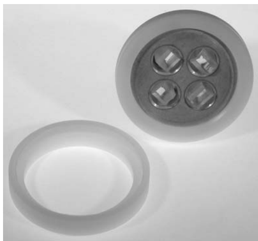
Fig. 10. Holder with four epoxy tablets clamped in place (top) and replacement plastic ring
