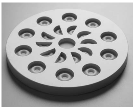
Fig. 23. Silicone rubber mold produces half- and full-disk forms.
