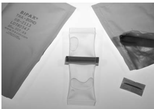
Fig. 6. Tra-Bond 2113 epoxy packaging. Epoxy is sealed in dated foil pouch (open at right), with silica gel packet.
