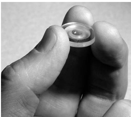
Fig. 22. Polished disc for easy production of single high-quality embedded samples.
