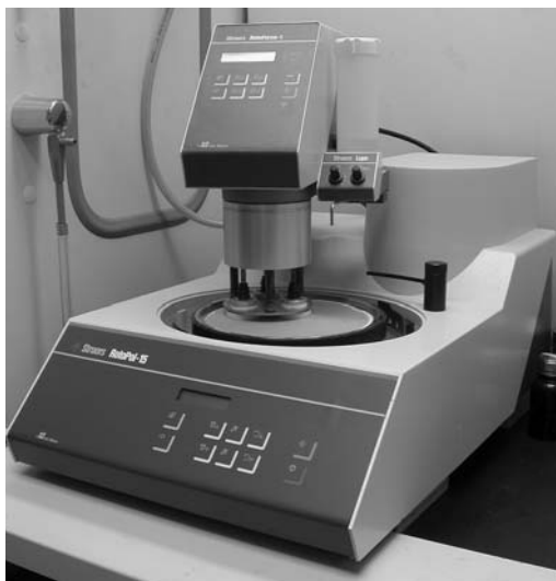
Fig. 17. Semiautomatic polisher (based on Struers RotoPol-15) for processing up to 12 samples in three holders simultaneously
