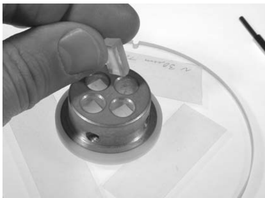
Fig. 12. Holder inverted on glass plate for registration of embedded samples. Adhesive tape on glass advances tip beyond ring edge prior to polishing (here, approximately 30 \mu\text{m} ).
