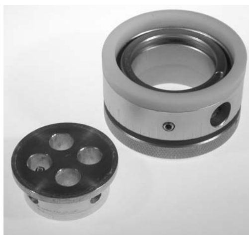
Fig. 11. Holder, without ring, can be used in Struers Accustop. This calibrated fixture (20 \mu\text{m} divisions) allows removal of measured amounts of material.
