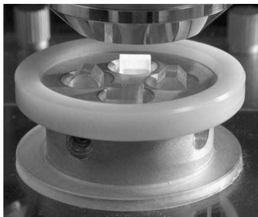
Fig. 20. Holder under 10x bright-field/dark-field objective. Since the sample surface and ring are parallel to the base of the holder, all samples are flat and in the same plane. The holder can be rotated to the next sample without losing focus or damaging objectives during rotation.
