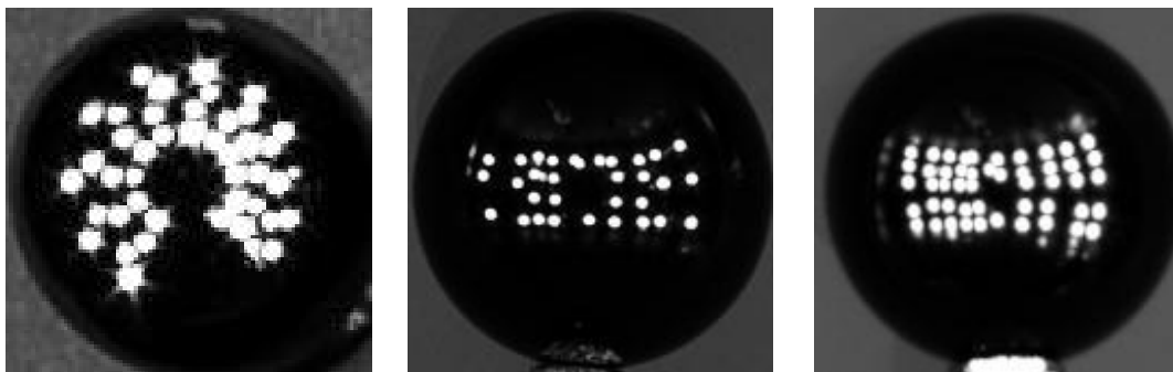
Figure 3 (left) The highlights on this reference sphere illustrate a near ideal setup with even coverage and an almost complete hemisphere of light with the exception of where the studio stand is located. Figure 4 (middle) The reference sphere for a wall-hung painting shows the restrictions of the studio size and ceiling height. The reflections create more of a bow tie pattern as compared to Figure 3. Figure 5 (right) The reference sphere for a wall-hung object with reflections from the walls, ceiling and floor (the less defined reflections).
