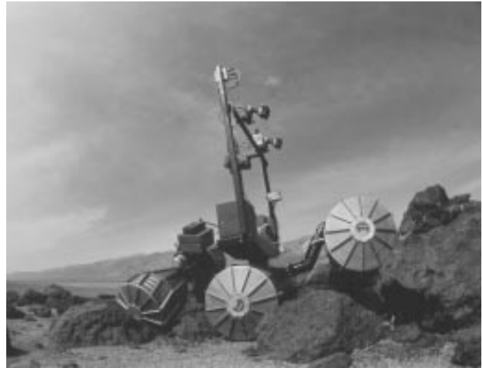
This Russian Mars Rover maneuvers the rough terrain of Death Valley, California, by following detailed instructions programmed into its onboard computer. More elaborate versions of such a robot might help build a base on Mars.
