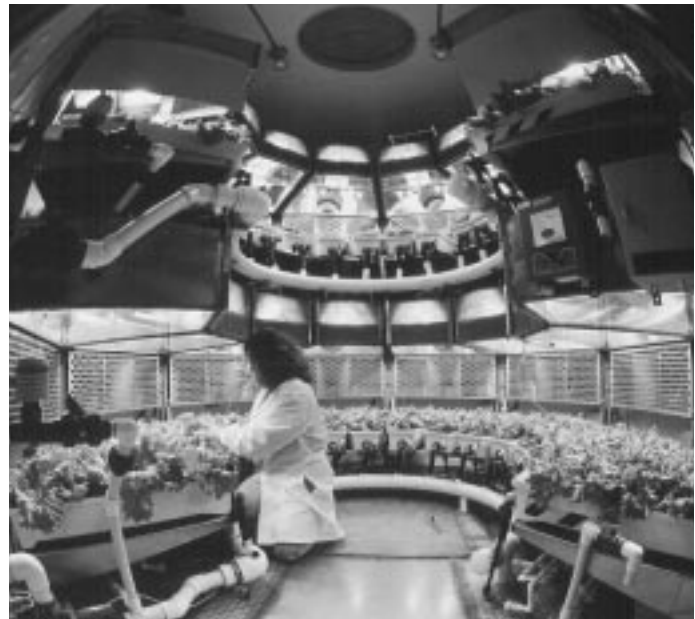
Scientists study the challenges of maintaining closed systems by growing plants in this room which can be sealed so that nothing but energy enters or leaves.
