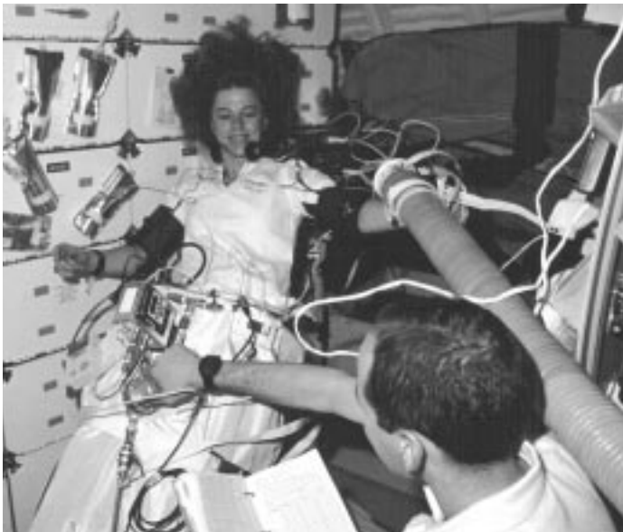
Shuttle astronauts study how weightlessness affects humans. Here, Bonnie Dunbar is wearing a device that pulls body fluids toward her feet. David Low monitors the test.
